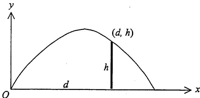
A stone is projected from a point on the ground, and it just clears a fence  $d$  metres away. The height of the fence is  $h$  metres. The angle of projection to the horizontal is  $\theta$  and the speed of projection is  $V$  m/s.
